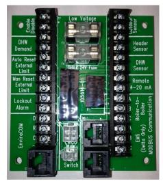
For Boiler to Boiler use either RJ45 Ethernet cable in one of the plugs on the PCB and plug the other end into the next boiler. Or, you have a choice to hardwire ABC of the boiler to boiler lugs. If you are using a BMS you must also hardwire ABC on the EMS lugs as well, daisy chaining to the other boilers.
