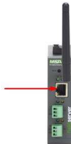
Figure 3-4: ProtoAir Ethernet TCP/IP and BACnet IP Connection
