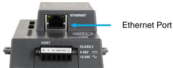
Figure 9: Ethernet port location on the ProtoNode
