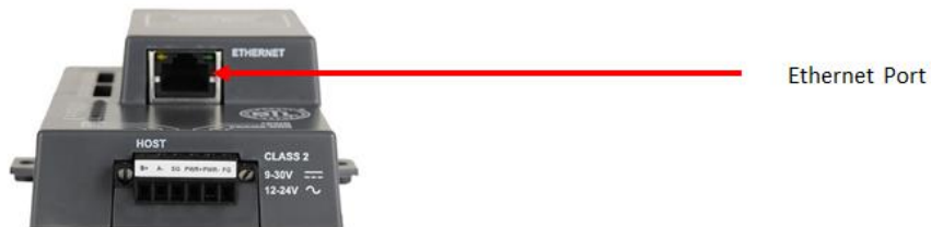
Figure 18: Ethernet port location of the ProtoNode
