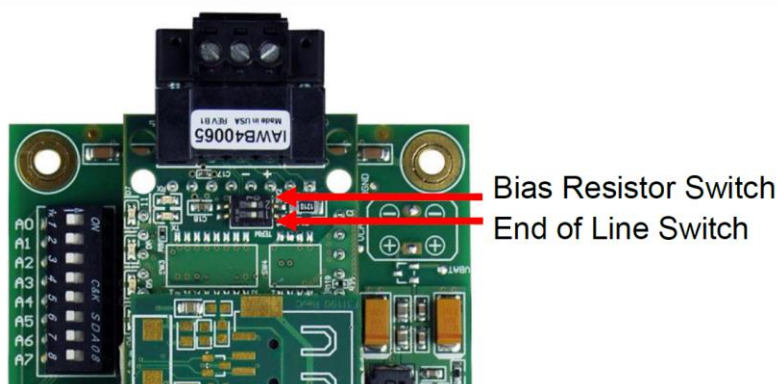
Figure 7: End-of-line termination on from ProtoNode to RS-485 Field Protocol –BACnet MS/TP or Metasys N2.
